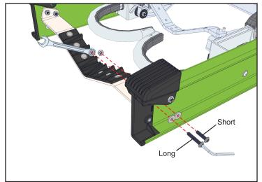
5. Align the new V-bar with the holes, then using a 1/8" Allen wrench and 3/8" wrench, tighten the new fasteners in the order shown. Make sure the long screw is closest to the end of the rail.
