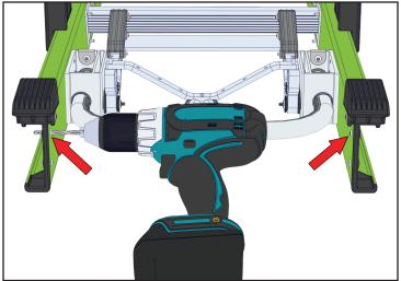
3. Using a drill and 13/64" bit, drill completely through the center of the rivets next to the wall pads.
