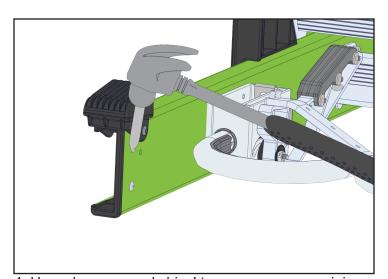
4. Use a hammer and chisel to remove any remaining rivet head material. Be careful not to damage the fiberglass rail.
