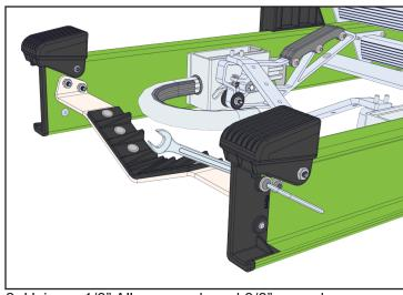
2. Using a 1/8" Allen wrench and 3/8" wrench, remove and discard the old V-bar and hardware. Move ahead to step 5.
