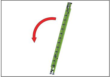
1. Lay the ladder down with the fly section facing the ground. If the V-bar is being added to the ladder skip to step 3.
